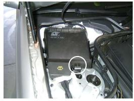
1. The filter is located under the hood below the windshield on the passenger side. Remove the 10mm plastic nut that secures the filter box. Pull up slightly to remove the filter box.
