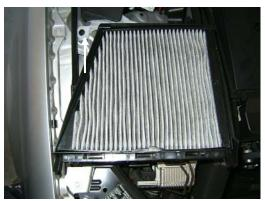
2. Flip the filter box over, remove old filter by pulling it up.
