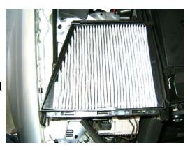
3. Insert new TYC filter into filter box, ensuring that the Air Flow arrow is pointing up. (It will point down later as you flip the box to reinstall)
