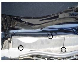
1. The filter is located under the hood, at the passenger side. Locate the 3 retaining pins securing the cowl cover. Remove the pins.
