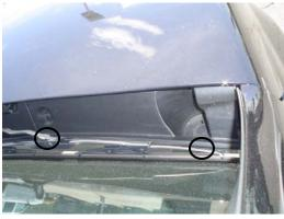
2. Directly below the wiper at the bottom of the windshield, locate the additional 2 retaining pins that secure the cowl cover. Push up cowl cover to expose the filter housing under it.
