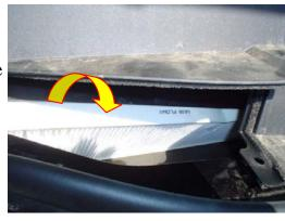
3. Pull out slightly and slide up the old filter to remove it. Replace with new TYC filter, ensuring that the Air Flow arrow is pointing to the vehicle's cabin.
