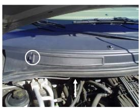
1. The filter is located under the hood, near the passenger side. Locate the filter access door and push on the locking tab to remove it. Set door aside.
