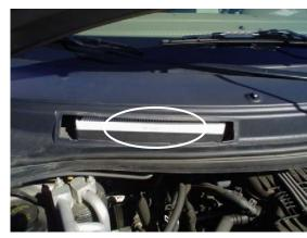
3. Replace with new TYC filter, ensuring that the Air Flow arrow is pointing down.
