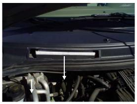
2. Push up slightly on the filter from its tray and slide it out to remove.
