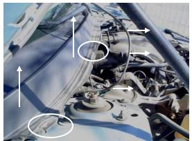
1. The filter is located under the hood, near the passenger side. Pull away the hose running along the cowl cover. Remove the 2 clips that secure the cowl cover and pull the entire cover up.
