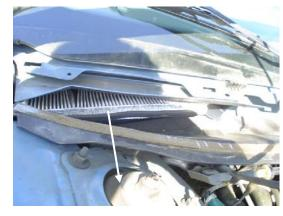
2. After removal of cowl cover, filter will be visible. Push up slightly on the filter from its tray and slide it out to remove.
