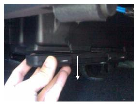
2. Pull down the loose filter access door to expose the filter inside. Set filter access door aside.
