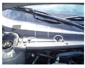
1. The filter is located under the hood, below the windshield on the passenger side. Open the filter cover by pushing on the 2 retaining tabs and then pulling the cover up.
