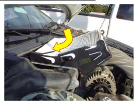
3. Remove old filter from its frame. Install new TYC filter, ensuring that the Air Flow arrow is pointing down.
