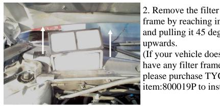
frame by reaching in and pulling it 45 degree upwards. (If your vehicle does not have any filter frame, please purchase TYC item:800019P to install)
