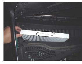
3. Remove old filter by sliding it up. Insert new TYC filter, ensuring that the "Rear of car" arrow is pointing towards the back of the car.
