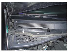
2. Flip down on the filter access door to expose the filter sitting inside. \*
