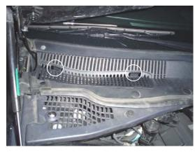
1. The filter is located under the hood, under the windshield on the passenger side. Push on the 2 tabs to remove the plastic cover.
