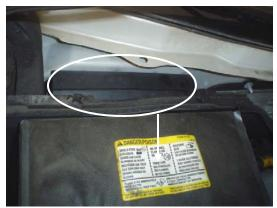
1. The filter is located under the hood below the windshield at the passenger side. Pull away the rubber lining and remove the 4 bolts securing the plastic cowl cover. Lift up and remove cowl cover, set it aside.
