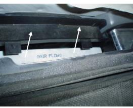
3. Slide out the old filter from its housing and replace with new TYC filter. Ensure that Air Flow arrow is pointing towards the cabin of the vehicle.
