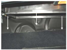
1.The filter is located below the glove compartment, at the passenger side kick panel. Remove the plastic cover by pulling it downwards.
