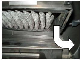
2. The filter will be visible once the cover is pulled down. Pull down old filter and slide to the right to remove. Note: Filter is installed in a curved position in the vehicle.
