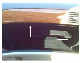
1. The filter is located behind the glove compartment. Open the glove box, lift up shelf and pull to the left to release.
