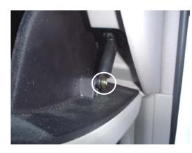
2. Locate retainer arm on the right bottom of the glove box, unscrew to disconnect it. Allow glove box to swing down on its hinges, exposing the filter behind it.
