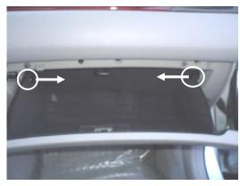
1. The filter is located behind the glove compartment. Twist the removable latches on each side of the glove box, and remove them by pushing them inwards.
