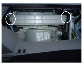
3. Push on the 2 retaining tabs to release the filter frame. Slide out the filter frame. Replace old filter in frame with new TYC filter, ensuring that the Air Flow arrow is pointing down.
