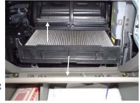
3. Slide out filter frame, remove old filter and replace with new TYC filter. Ensure that Air Flow arrow is pointing down.
