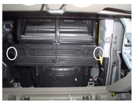
2. Filter access door will then be visible. Push on the 2 retaining tabs on the sides to release the door.
