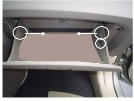
1. The filter is located behind the glove compartment. Push in on the retaining latches to remove them. Remove the retainer string attached to the glove box. Allow glove box to swing down on its hinges.
