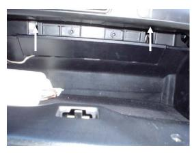
1. The filter is located behind the glove compartment. Open glove box, remove plastic cover piece by sliding it upwards. This allows access to the filter access door.
