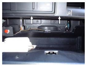
2. Pull up on the filter access door to release it . Remove and set door aside.
