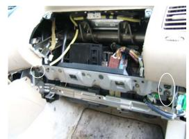
3. Remove the metal support beam by removing the 3 screws that secure it.
