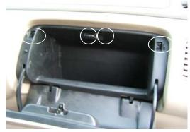
1. The filters are located behind the glove compartment. Remove the 4 screws that secure the glove compartment.
