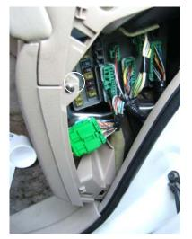
2. Remove the panel beneath the glove compartment by removing the screw in the fuse box.
