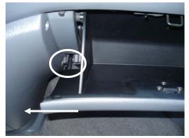
1. The filters are located behind the glove compartment. To remove the glove box, disengage the hinge on the left side by pulling the glove compartment upwards. After the left hinge is loose, slide the entire box to the left to dislodge the right hinge.
