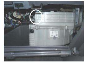
2. After the glove box is removed, the filter access door is visible. Pull on the locking tab on the left to remove the door, exposing the filters inside. Note: This application contains 2 identical filters.
