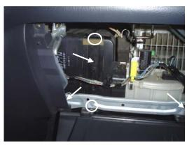
2. Remove the 2 bolts at the bottom securing the metal cross bar. Pull on the top and bottom tabs to release the filter access door. Remove door and set it aside.
