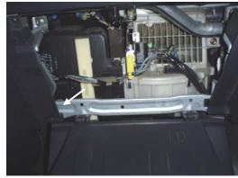
3. Slide out the old filter and replace with new TYC filter, making sure Air Flow arrow is pointing to the driver's side.
