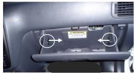
1. The filter is located behind the glove compartment. Push in on the sides while pulling down to disengage the latches. Allow glove box to swing down on its hinges, exposing the filter access door behind it.
