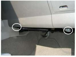
2. Identify and remove the remaining 2 screws at the bottom of the glove compartment. Remove compartment by pulling it outwards. This exposes the filter access door behind it.
