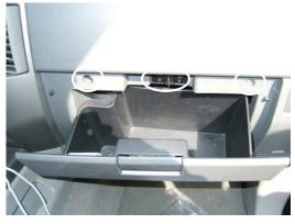
1. The filters are located behind the glove compartment. Remove the screws at the top of the glove compartment.
