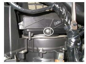
3. Remove the single bolt that secures the filter access door. Remove door and set it aside. Slide out old filters, replace with new TYC filters. Ensure that the Air Flow arrow is pointing down for both filters.
