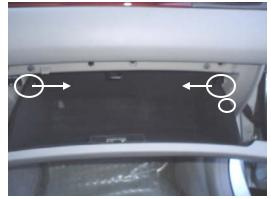
1. The filter is located behind the glove compartment. Remove the latches by pushing them inwards. Remove the damping mechanism at the right side of the glove box door. Allow glove box to swing down on its hinges, then remove glove box by pulling it out.
