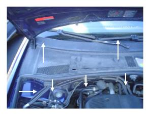
1. The filter is located under the hood at the passenger side. Pull away the rubber lining found at the end of the cowl cover, and lift it up. Filter is located under the cowl cover.
