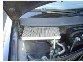
3. Pull up filter and slide it out. Replace with new TYC filter. Ensure that Air Flow arrow is pointing down.
