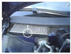
2. Pull up on the plastic hook that secures the old filter in place and set hook aside.
