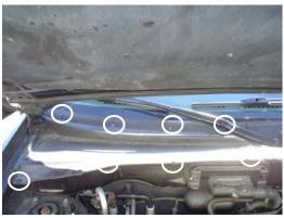
1. The filter is located under the hood, below the windshield on the passenger side. Remove the 4 plastic retainers and 4 screws to loosen the cover.
