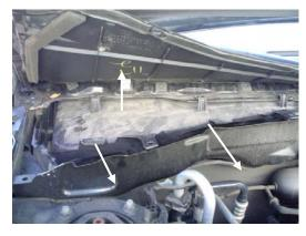
2. Lift up the plastic cover to expose the filter cover. Lift up filter cover and slide it out.
