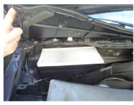
3. Remove old filter from the tray, insert <u>new TYC filter</u> in its place. Ensure that the Air Flow arrow is pointing down.
