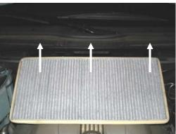
3. Slide <u>new TYC filter</u> into cavity. Ensure that Air Flow arrow is pointing down.
