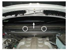
1. The filter is located under the hood, under the windshield. Locate and loosen the 2 screws securing the filter cover, lift up the cover to expose the filter under it.
