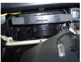
3. Slide out old filter (if present\*) and replace with new TYC filter. Ensure that Air Flow arrow is pointing down.
