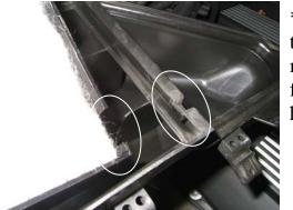
\*NOTE: When installing the new filter, be sure to match up the notch on the filter and the filter housing.
