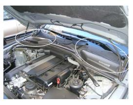
1. The filters are located in the engine bay, with one on each side, below the windshield.
