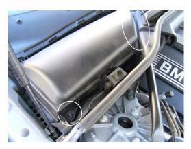
2. Remove filter holder by unclipping the metal bar and loosening the plastic clip.
