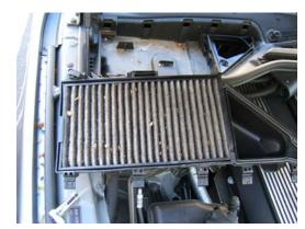
3. Slide filter holder forward to remove. Remove old filter from its holder and install new TYC filter. Ensure that Air Flow arrow is pointing down.\*
