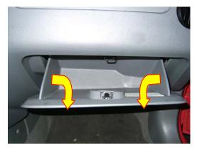
1. The filter is located behind the glove compartment. Open glove box and push on the sides while pulling down to disengage the latches. Allow glove box to swing down on its hinges.
