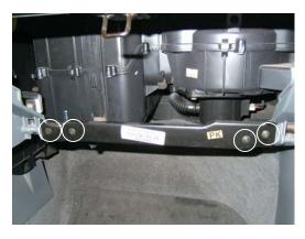
2. Remove the 4 screws securing the metal support bar, and remove the entire bar.
