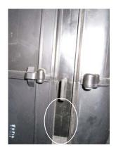
\*NOTE: Please note the installation direction on the frame when installing the filter. The arrow should be pointing upwards.
