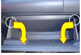
1. The filter is located behind the glove compartment. Open glove box and push in on the sides while pulling down to disengage the latches.
