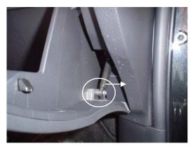
2. Locate retaining arm on the bottom right of glove box, pull arm towards the right to release. Allow glove box to swing down on its hinges, exposing the filter access door behind it.
