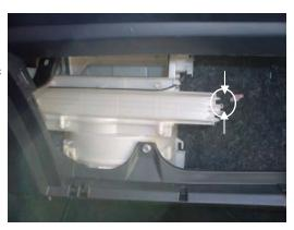
3. Push on the retaining tab to release the filter access door. Remove door and set aside.
