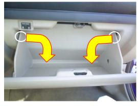
1. The filter is located behind the glove compartment. Open glove box and push on the sides while pulling down to disengage the latches.
