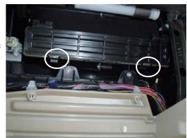
3. Pull on the 2 retaining tabs on the filter access door. Remove door and set it aside.
