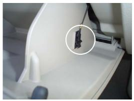
2. Unhook the string that is secured on the plastic hook on the right side of the glove box. This allows the glove box to swing down and expose the filter access door behind it.
