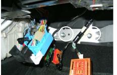
3. Remove 2 x 12mm nuts that hold the junction box bracket and remove bracket.
