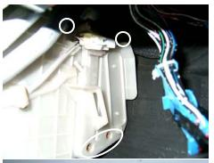
4. Remove 4 screws on the filter access door and unplug the harness on the filter access door.
