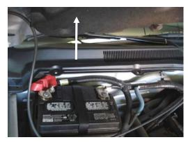
2. Lift up the plastic cowl cover to access the filter housing under it.
