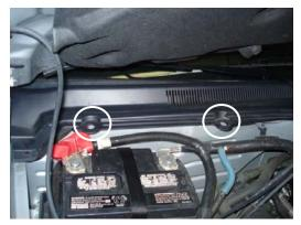
1.The filter is located in the engine bay right below the windshield on the passenger side. Remove the 2 clips securing the plastic cowl cover in place.
