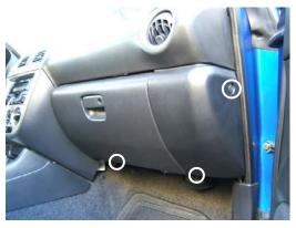
1. The filter is located behind the glove compartment. Remove 1 clip on the side and 2 screws beneath the compartment.
