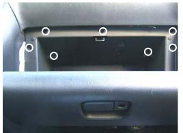
2. Remove 7 screws to remove glove compartment.
