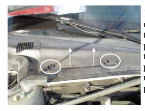
1. The filter is located under the hood, below the windshield at the passenger side. Open the filter cover by pushing on the 2 retaining tabs and then pulling the cover up.
