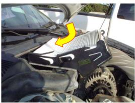
3. Insert <u>new TYC filter</u> and frame back into vehicle at a 45 degree angle.
