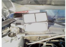
2. Remove the filter frame by reaching in and pulling it 45 deg upwards. If your vehicle does not have any filter frame, skip this step and proceed to step 3.\*
