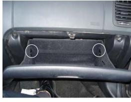
1. The filter is located behind the glove compartment. Remove the latches on each side of the glove box by pushing them inwards. Allow glove box to swing down on its hinges.
