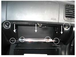
2. Remove the bolts and screws holding the back panel of the glove box in place. Pull down the entire panel to expose the filter access door behind it.
