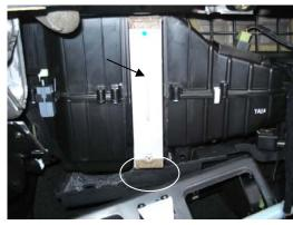
3. Remove the vertical filter access door by unlatching the bottom of the door and pulling it out. Slide out exposed filter and replace with new TYC filter. Ensure that Air Flow arrow is pointing to the driver's side.
