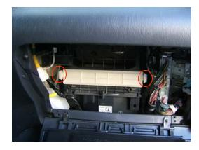
2. Push on the 2 locking tabs found on the filter access door and slide out the filter tray.
