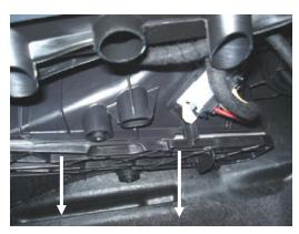
2. The filter is housed within the plastic filter access door shown. Pull down on the door to remove it. Set door aside.
