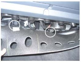
1. The filter is located below the glove compartment. Pull down the foam cover sheet to expose 2 plastic screws that secure it in place. Using a flat-head screwdriver, remove the screws and pull off foam cover.
