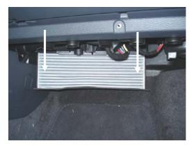
3. Remove the old filter by sliding it downwards. Insert new TYC filter by sliding it up into the old filter's position. Ensure that Air Flow arrow is pointing to the vehicle's cabin.
