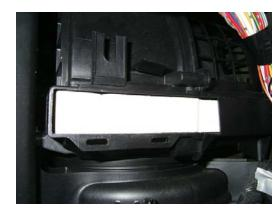
3. Slide out old filters and install new TYC filters. Ensure that Air Flow arrow is pointing down for both filters.
