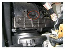
2. Remove the filter access door by lifting up the locking tab. Set door aside.
