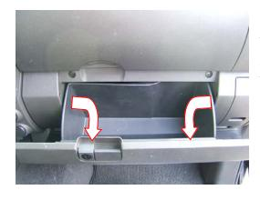
1. The filters are located behind the glove compartment. Open glove box and push on the sides while pulling down to disengage the latches.
