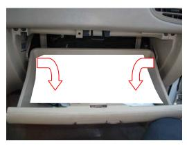
1. The filter is located behind the glove compartment. Open the glove compartment, push on the sides while pulling down to disengage the latches. Allow the glove box to swing down on its hinges.
