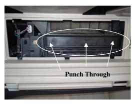
2. The filter is optional and may not be installed in all vehicles\*. If the filter compartment is sealed as shown, use a flat head screwdriver to punch through the perforated plastic cover.
