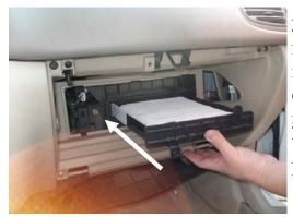
3. Remove the old filter frame (if present) by sliding it out towards you. Remove old filter from its frame and install new filter, ensuring that Air Flow arrow is pointing down.
