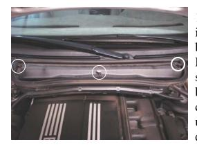
1. The filter is located inside the engine bay, below the windshield. Remove the 3 clips securing the filter cover by turning them counter-clockwise. Lift up the plastic cover to expose the filter under it.
