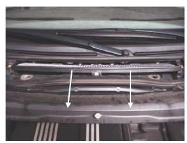
2. Remove old filter by lifting it off the slot and sliding it out. Slide into place <u>new TYC filter</u>, ensuring that Air Flow arrow is pointing down.
