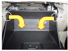
1. The filter is located behind the glove compartment. Push on the sides while pulling down to disengage the latches. Allow glove box to swing down on its hinges. Filter access door will now be accessible.
