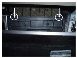
2. Push down on the 2 retaining tabs to remove the filter access door.
