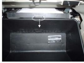
3. Grab the handle of the filter tray and slide it out. Remove old filter from tray and replace with new TYC filter.
