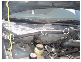
1. The filter is located in the engine bay, under the windshield on the passenger side. Locate the 3 clips holding the plastic cover in place and remove cover.
