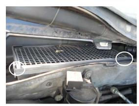
2. Release filter cover by pulling on the 2 locking tabs. Remove filter cover.
