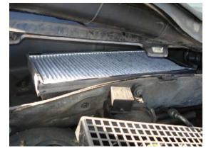
3. Insert <u>new TYC filter</u> into the space where the cover used to be. Ensure that the Air Flow arrow is pointing down.
