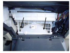
3. Slide out filter frame, remove old filter and replace with new TYC filter.
