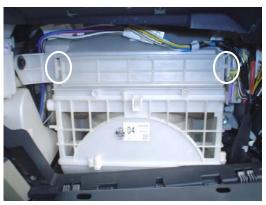
2. Filter access door will be visible after the glove box is swung open. Push on the 2 plastic tabs to release the filter access door.
