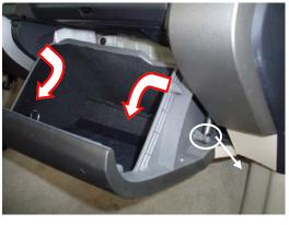
1. The filter is located behind the glove compartment. Push in the sides of the glove box to disengage the latches and allow it to swing down. Pull on the retaining arm on the right side of the glove box to release it.
