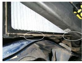
2. Remove filter and filter holder by releasing the 2 locking tabs on the filter holder.
