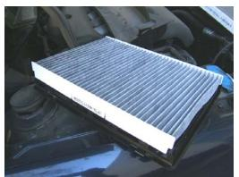
3. Remove old filter and <u>install new TYC filter</u>, ensuring that the Air Flow arrow is pointing down.
