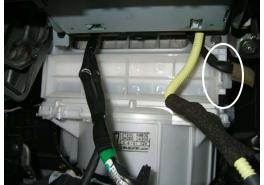
3. Remove the filter access door by pushing on the locking tab to release it.
