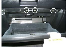
2. Open glove compartment and remove the 4 screws securing the compartment. Remove compartment and set aside.
