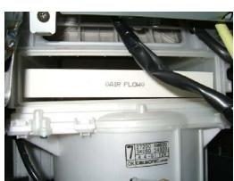
4. Slide out old filter and <u>install new TYC filter</u>. Ensure that Air Flow arrow is pointing down.
