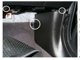
1. The filter is located behind the glove compartment. Remove plastic panel under the compartment. Remove plastic nut securing the kick panel. Remove two screws under the glove compartment.
