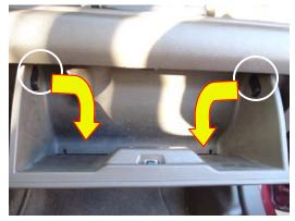
1. The filters are located behind the glove compartment. Push on the 2 black retaining latches on the glove box to remove. Let glove box swing down on its hinges and expose the filter access door behind it.
