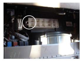
2. Pull on the tab on the filter access door to release it. <u>Set filter access</u> door aside.
