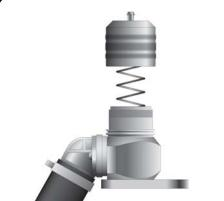
Remove the spring-loaded cap with caution. Remove the spring but do not remove any other components.
