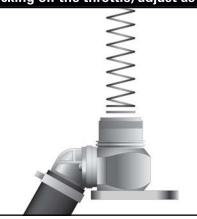
Insert one adjustment washer beneath the spring and replace cap
