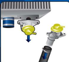
Remove the factory bypass valve from the front of the factory intercooler and disconnect the recirculation hose
