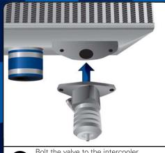
Bolt the valve to the intercooler using the supplied bolts, taking care not to damage the gasket
