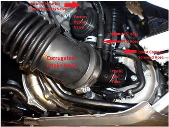
1. Remove the plastic undertray from the car to get access to the Factory Bypass Valve.
