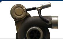
Connect SBC to pressure source and wastegate actuator
