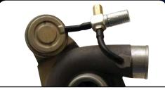
Connect HPBC to pressure source and wastegate actuator
