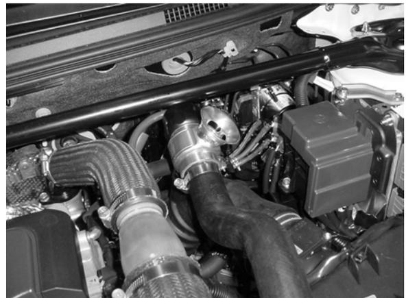
**Note:** The Dual port is supplied with a blanking plug for the vent to atmosphere side of the BOV to convert the BOV to full recirculation mode. Simply unscrew the trumpet and screw in the supplied blanking plug. Alternatively, the blanking plug can be used to convert the BOV into full vent to atmosphere mode by installing the blank onto the plumb back side. An additional 34mm hose blank (sold separately) is required to block off the plumb back hole in the intake pipe.
