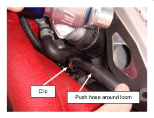
5. Refit the BOV using the standard screws. Start the engine and check for leaks.
