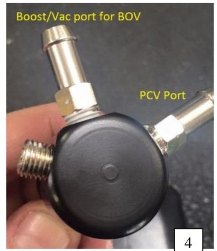
5. Install Boost Reference Adapter on to the PCV fitting on the intake manifold and install the retaining clip. Hook up the PCV with the supplied 130mm PCV hose to the lower fitting, also install the supplied 5mm vacuum hose to the other post as shown below. Use slotted hose clamp and spring clamp to secure each hose in place respectively.
