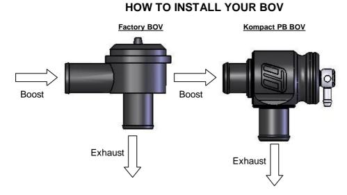
Note: Be sure to mount the Kompact plumb back in the orientation shown above compared to the standard BOV.
